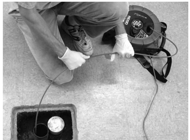
Figure 24 – Proper Technique For Pushing Cable Back Into Drum
