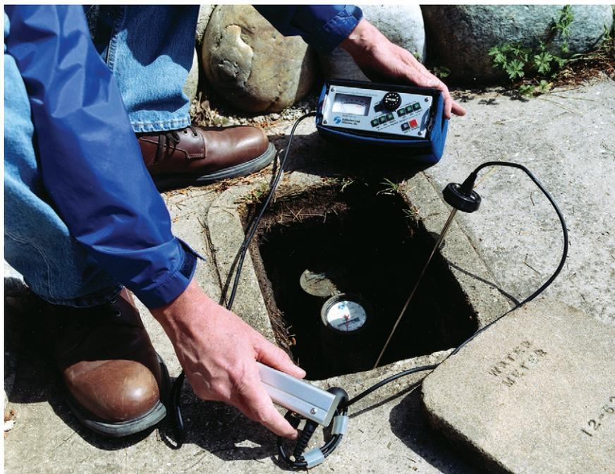
*Figure 4-8 Leak Survey at a Meter*
