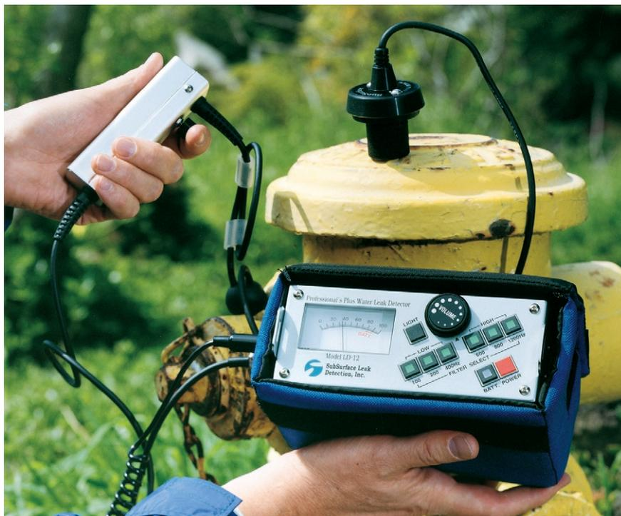
*Figure 4-6 Leak Survey at a Hydrant*
