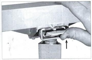
3. Lock the cradle tilt latch and lift the cradle off of the frame.
