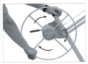
4. Rotate the winch forward one full rotation.
