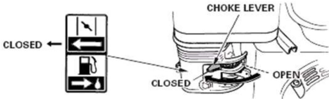
Once the engine is started, move the choke to the OPEN position (**to the right**)
