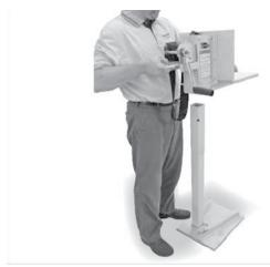
3. Let out a 2' loop of strap on the Collar Assembly and slide the Collar Assembly over the Boom Tube. **MAKE SURE** the seat of the Collar Assembly is oriented on the same side as the Counter Base as shown.
