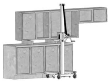
1. Start by using the Dolly Base Assembly to raise the upper cabinets to blocks (approx. 9" high, blocks not included) on the base counters.
