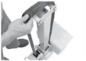
5. Position the strap over the top rollers, making sure that it is aligned straight with no twists.
