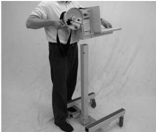
3. Let out about a 2' loop of strap on the Collar Assembly and slide the Collar Assembly over the boom tube.
