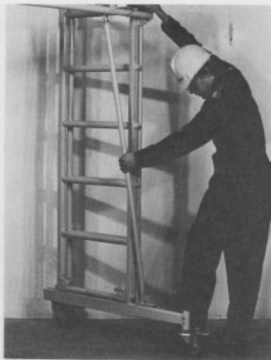
With latch pin disengaged, adjust outrigger position by raising end section slightly and sliding outrigger in or out with foot.
