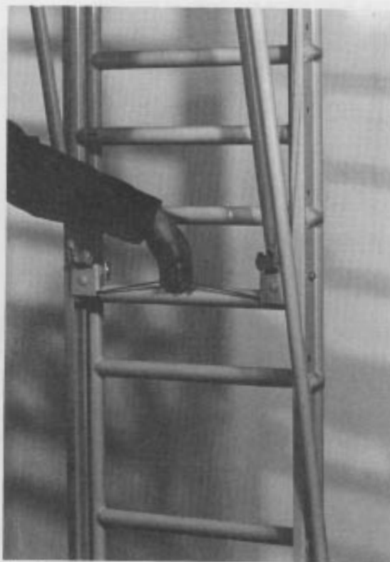
If ladder lock spring pins do not readily engage, raise cable between sheaves slightly and jog telescoping ladder section.
