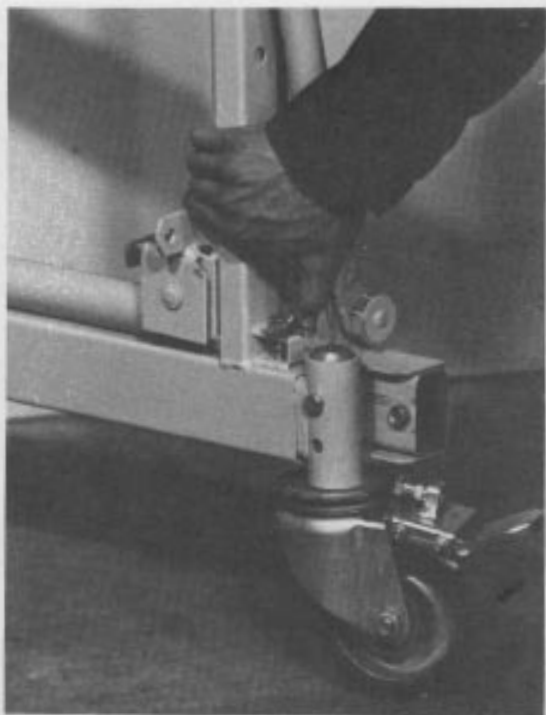
Latch pins hold outriggers in either fully extended or fully retracted positions. Raise and rotate to disengage.
