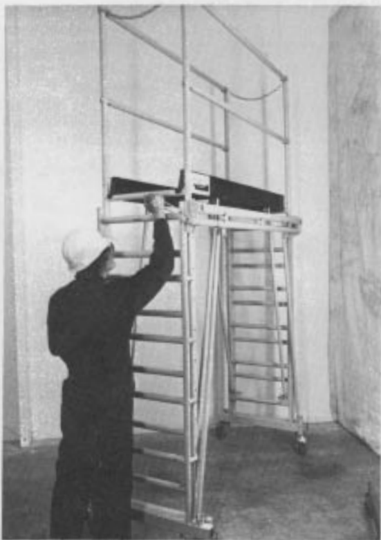
TO ELEVATE DECK— Retract & rotate ladder lock spring pins to disengaged position.
