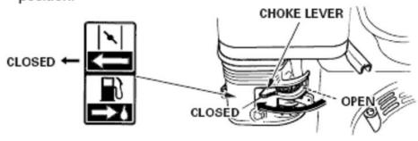
To restart a warm engine, leave the choke lever in the OPEN position.
