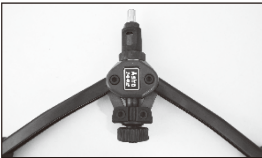
Riveter properly prepared for setting rivet nuts
