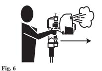
Apply steady downward pressure to the handles and apply enough throttle to engage the clutch and hammer.
