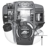
Upper limit of engine oil. Lower limit of engine oil is end of dipstick.
