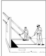
When the wall reaches the upright position, it is stopped and held firmly by the preset wall stops, which are adjustable.
