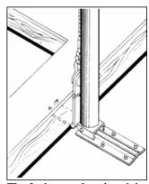
The Jacks are placed upright, flush against the lifting bracket. The hinged foot is securely nailed to the subfloor near a floor joist.
