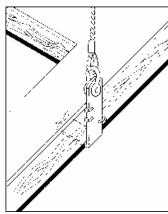
The lifting brackets are placed under the top plate or header and securely nailed. The bottom of the wall is secured with metal strapping to prevent it from slipping during the lift.
