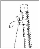
The adjustable wall stops must be pre-set at approximately 1.45 times the wall height.
