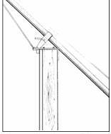
The Wall Jacks provide a substantial brace until the wall can be permanently braced with the Proctor Adjustable Wall Braces.
