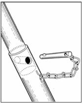
A minimum of two Proctor Wall Jacks must be used for any wall lift. (We furnish them in pairs.) Pin the tubes in the extended, working position.
