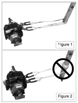
ACAUTION AVOID INSTALLING THE SLING ON SHARP EDGES THAT MIGHT DAMAGE IT. WHETHER YOU ARE USING A POST, A TREE OR A STUMP, ALWAYS INSTALL THE SLING NEAR THE ANCHOR'S BASE (FIGURE 1).
