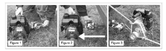
NOTE: Do not leave the winch on the hitch with the engine running; the resting position will cause the Oil Alert device to turn the Honda engine off.
