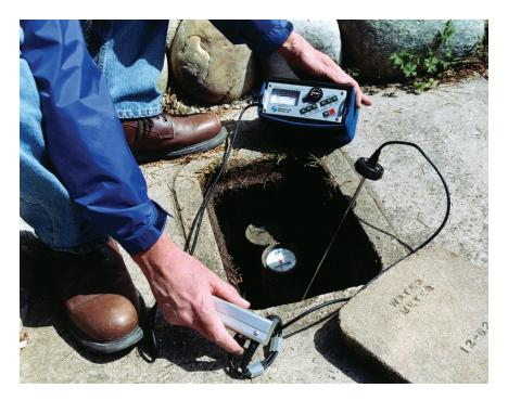
Figure 4-8 Leak Survey at a Meter
