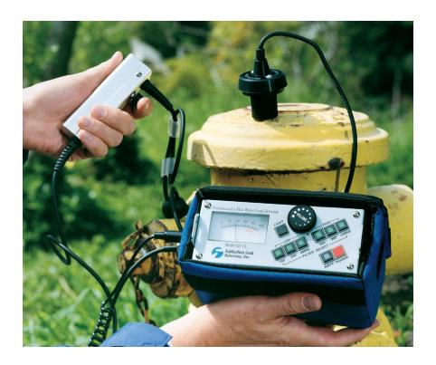
Figure 4-6 Leak Survey at a Hydrant
