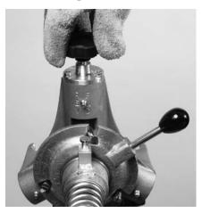
Continue to automatically feed cable until obstruction is met. When cable begins to drag or rotation becomes difficult, move the lever to the **NEUTRAL** position and allow tool to cut away at the obstruction. (See Figure #4 for **NEUTRAL** feeder position)
