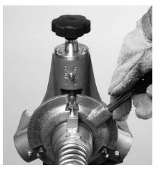
**DANGER: NEVER** force the cable or tool into the obstruction. Choose the proper feeding speed in order to give a smooth cutting action.
