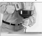
Tips: If you cannot get the cable through a trap, unscrew the clean-out plug. Be sure to put a pan under the plug before unscrewing. Insert cable into clean-out opening.
